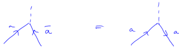
Fig. 9.5 Fusion of an anyon with its anti-anyon to form the identity can be thought of as a particle turning around in space-time.
