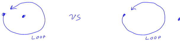
Fig. 19.2 To find the statistical phase, we compare moving a particle in a loop versus moving it in the same loop when another particle is inside the loop.
