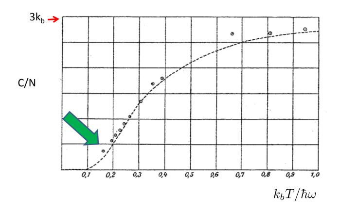
Low Temperature Heat Capacity of Diamond
