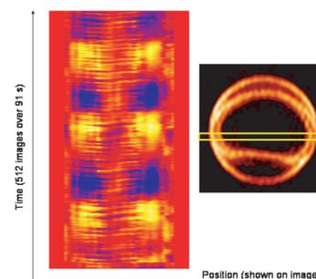
Figure 5: (left) Time progression of the shear layer at  $Re\sim 1800$ . (right) waves in the shear layer.
