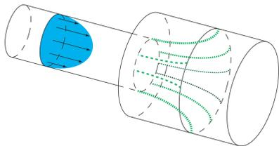
Figure 1: Schematic of the sudden expansion.
