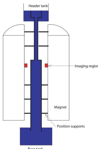
Figure 2: Schematic of the MRI visualisation system.
