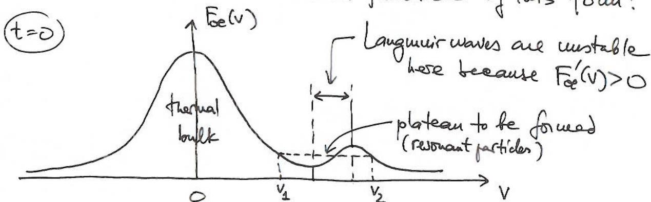
$$\boxed{\frac{\partial}{\partial t} |\vec{E}_k|^2 = 2\gamma_k |\vec{E}_k|^2}, \quad \gamma_k = \frac{\pi}{2} \frac{\omega_k^3}{k^2} \frac{1}{n_{oe}} F'_{oe}\left(\frac{\omega_k}{k}\right) \quad (45)$$
