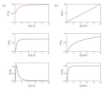
The internal energy U, the entropy S and the heat capacity  $C_V$  for (a) the twostate system (with energy levels  $\pm \Delta/2$ ) and (b) the simple harmonic oscillator with angular frequency  $\omega$ .
