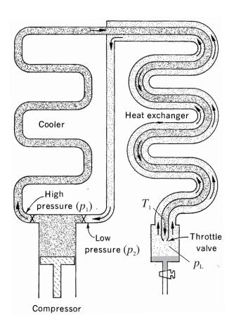
An advantage of the Joule–Kelvin liquefier is that the lower the temperature, the larger the drop in temperature for a given pressure drop. This is because the slope of the isenthalps increases as the temperature decreases (see curves for nitrogen on the previous page).
