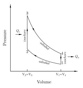
1.4 Show that the efficiency of the standard Otto cycle (shown above) is  $1 - r^{1-\gamma}$ , where  $r = V_1/V_2$  is the compression ratio.
