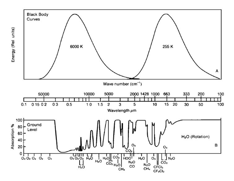
The upper figure shows the spectral energy density of thermal radiation from blackbodies at 6000 K and 255 K, corresponding to the average emitting temperatures of the Sun and Earth, respectively. The lower figure shows the percentage of the radiation incident on the upper atmosphere that reaches Earth's surface.
