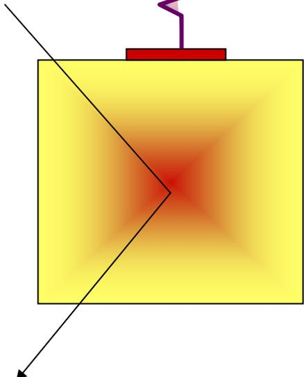
Particle interaction in absorber creates a temperature rise in thermometer which is proportional to energy deposition in absorber
