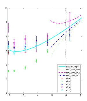
The discrete points are the lattice results, the solid lines are the corresponding Nambu-Goto energy levels, and other lines include the shifts we calculated from using the specific value  $c_4 = (D-26)/192\pi^2T^2$ . The vertical line is the expected radius of convergence for each level, we expect a matching only for points that are well to the right of this line.
