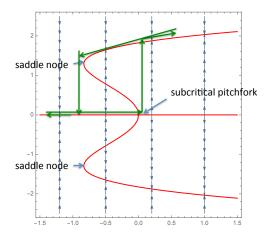
Figure 6: Stability diagrams for Equations (6) (top) and (7) (bottom) which contain subcritical pitchfork bifurcations.
