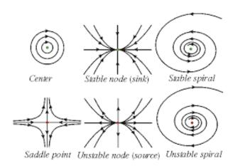
Figure 7: Fixed points in two dimensions.
