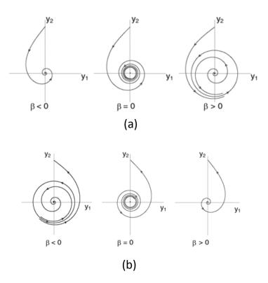
Figure 11: (a) Supercritical and (b) subcritical Hopf bifurcations.
