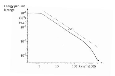
Figure 8: Scaling in the inertial subrange of bulk turbulence.
