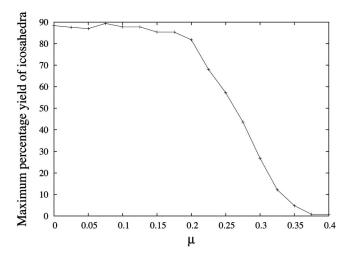
FIG. 10. The maximum yield of icosahedra as a function of the patch placement noise parameter  $\mu$ . In each case the yield is the average of five simulations at the values of T and  $\sigma$  which give the maximum yield for that value of  $\mu$ . Each simulation contains 1200 particles, at a number density of  $0.15\sigma_{1.}^{-3}$ .
