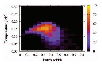
FIG. 11. (Color) Icosahedron yields using ring patches. The heat map shows the number of icosahedra formed after 80 000 MC cycles as a function of the patch width  $\sigma$  (measured in radians) and the temperature for 1200 particles at a number density of  $0.15\sigma_{LJ}^{-3}$ , using a single ring patch on each particle with  $\nu$ =1.017 rad.
