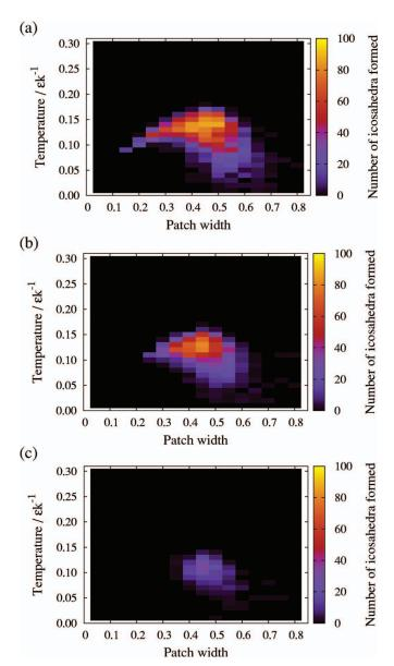
FIG. 9. (Color) The effect of noisy patch placement. The heat maps show the numbers of icosahedra formed after 80 000 MC cycles as a function of the patch width  $\sigma$  (measured in radians) and the temperature for 1200 particles at a number density of  $0.15\sigma_{\rm LJ}^{-3}$  for different noise levels in the patch placement: (a)  $\mu$ =0.1, (b)  $\mu$ =0.2, and (c)  $\mu$ =0.3.
