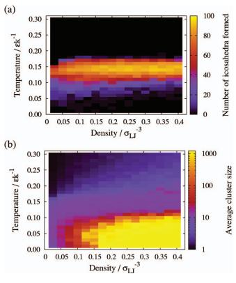
FIG. 8. (Color) (a) The number of icosahedra formed and (b) the mean cluster size (averaged over particles) after 80 000 MC cycles as a function of density and temperature for 1200 particles at a fixed patch width of  $\sigma$  = 0.45.
