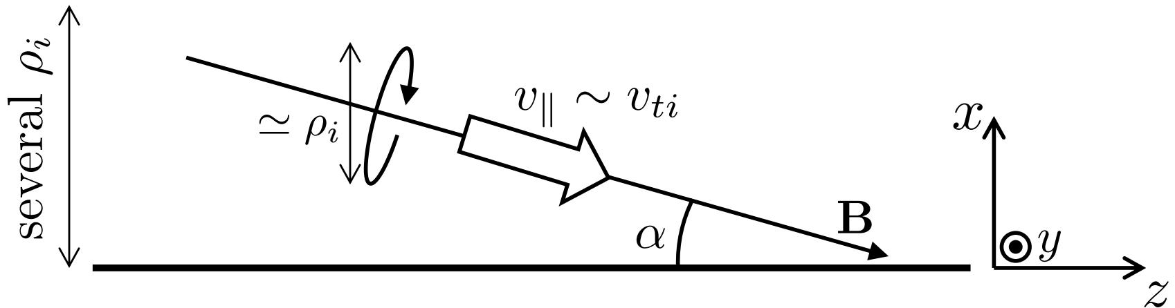
gyro-orbit time  $\sim \frac{1}{\Omega_i} \ll$  parallel streaming time  $\sim \frac{\rho_i/\alpha}{v_{ti}} \sim \frac{1}{\alpha\Omega_i}$
