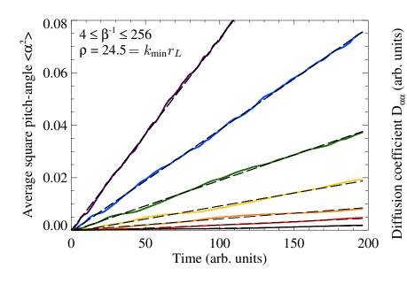
$$D_{\alpha\alpha} = \frac{3\pi}{8} \sqrt{\frac{3}{2}} \frac{e^2}{m^2 c^2} \left( \frac{\int_0^\infty k |\mathbf{B}_k|^2 \, \mathrm{d}k}{\int_0^\infty k^2 |\mathbf{B}_k|^2 \, \mathrm{d}k} \right) \frac{\langle B^2 \rangle}{\Gamma^2 v_{th}}$$
