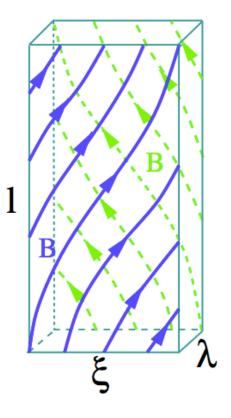
**Boldyrev 06**: eddies fully anisotropic;  $\xi/\lambda >>1$ ; become high-aspect ratio *current sheets* at small scales. (key idea: *critical balance + dynamic alignment*)
