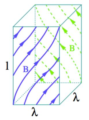
**Goldreich-Sridhar** (GS95): eddies' dimension perpendicular to the background field are comparable; become *filaments* at small scales. (key idea: *critical balance*)
