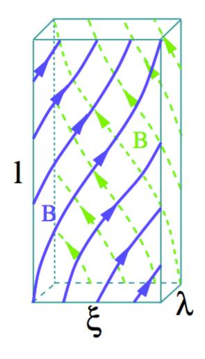
$$\begin{aligned} \xi \sim L(\lambda/L)^{3/4}, \\ \ell \sim L(\lambda/L)^{1/2}, \\ b \sim B_0(\lambda/L)^{1/4}, \\ \tau \sim \ell/V_{A,0} \sim \lambda^{1/2} L^{1/2}/V_{A,0}. \end{aligned}$$
