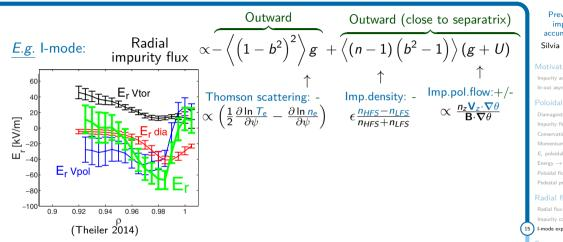
$\Rightarrow$  l-mode regime is favourable to avoid impurity accumulation, without invoking anomalous transport due to weakly coherent mode.
