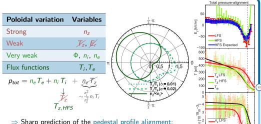
$\Rightarrow$  Sharp prediction of the pedestal profile alignment: total pressure with inboard impurity temperature.
