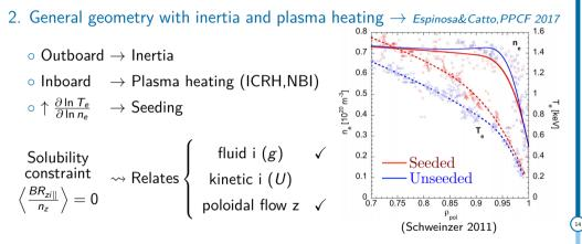
⇒ Solve the solubility condition for the kinetic effects, which cannot be measured, to express the radial impurity flux as a function of available diagnostics.
