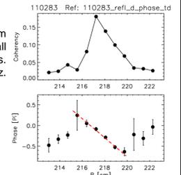
A linear phase shift is seen as a function of radius: similar to other measurements e.g. [6,7].
