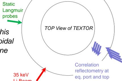
Measurements presented in this poster are performed at 3 toroidal locations in the equatorial plane + top of plasma
