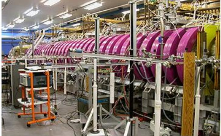
$$\begin{split} L &\sim 17 \ m, \ r \sim 0.5 \ m, \ B \sim 1 \ kG, \\ n &\sim 10^{12} \ cm^{-3}, \ T_e \sim 5 \ eV, \ T_i \sim 1 \ eV \end{split}$$
