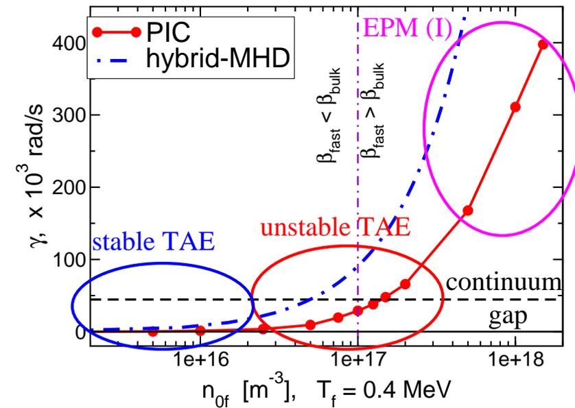
**TAE destabilized by fast particles. It is continuously modified into EPM as the drive increases.**
