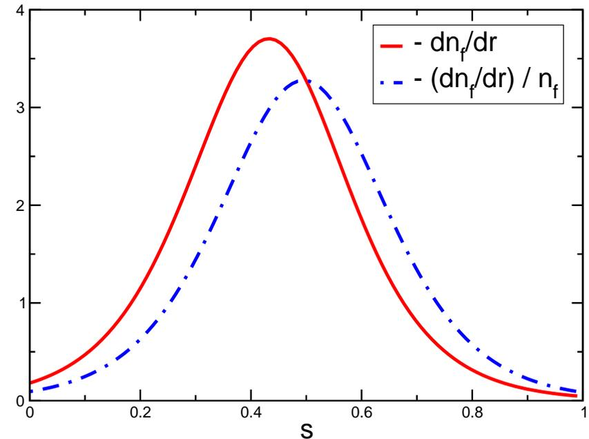
**Nonuniform fast-particle density is used to drive the modes**
