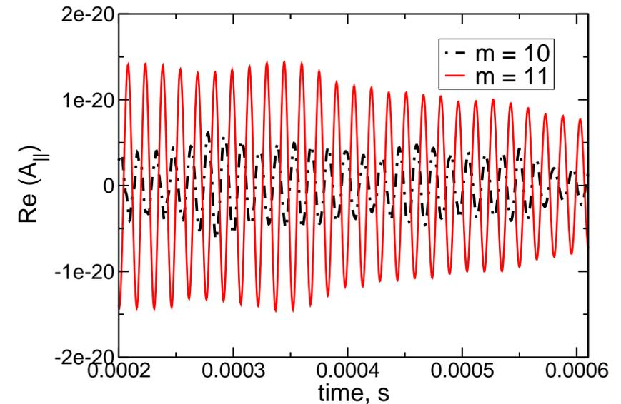
**Time signal resulting from the PIC simulations.**
