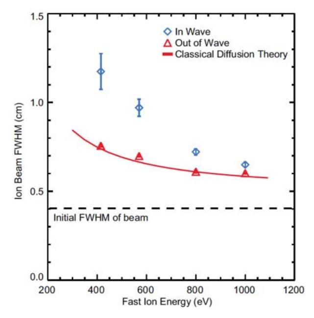
Beam spreading observed due to turbulence, increases with lower energy, consistent with orbit-averaging picture
