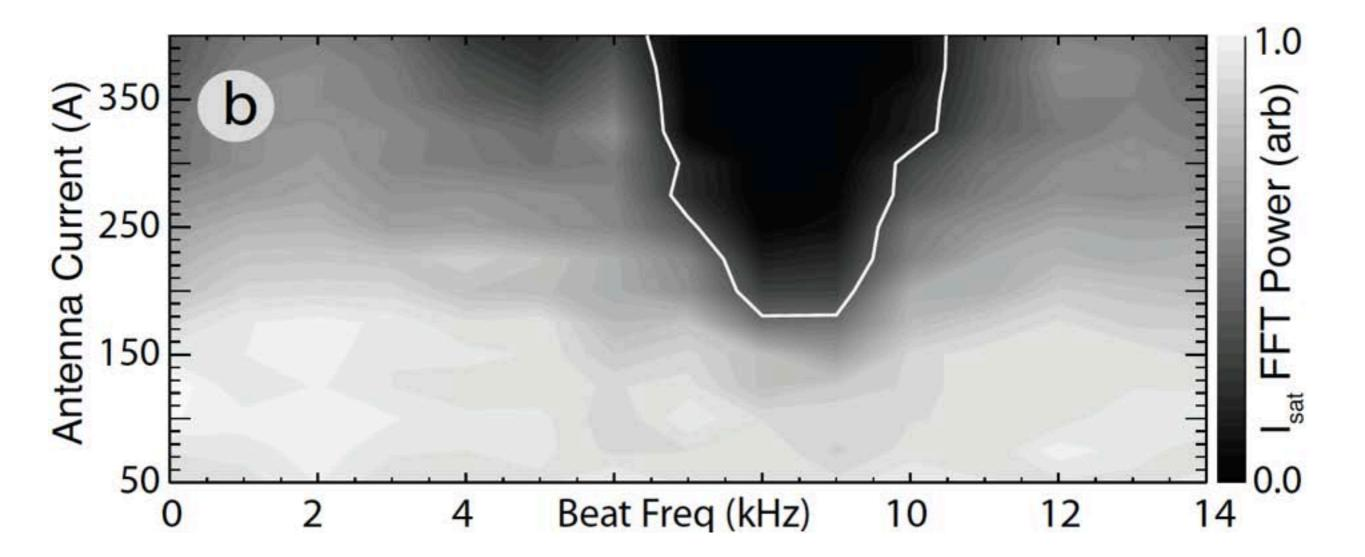
Window of mode stabilization/control increases with increasing BW drive
