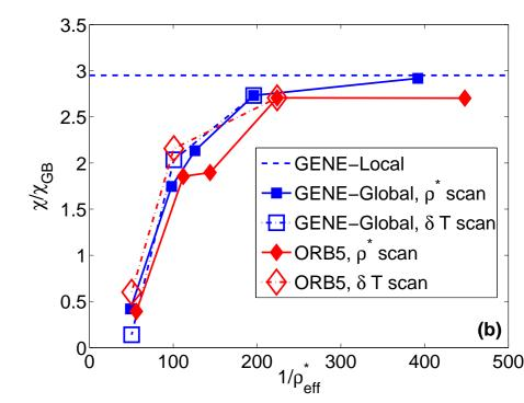
Heat diffusivity  $\chi_i$  in Gyro-Bohm units ( $\chi_{\rm GB} = \rho_s^2 c_s/a$ ) as a function of (a)  $1/\rho^* = a/\rho_s$  at fixed  $\Delta_T/a$ , and (b) as a function of  $1/\rho_{\rm eff}^* =$  $\Delta_T/\rho_s$  varying both  $\rho^*$  at fixed  $\Delta_T/a$  and  $\Delta_T/a$  at fixed  $\rho^*$ .
