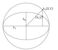
**Figure 1.0** The relation of input and output vectors of a  $2 \times 2$  Hermitian matrix with positive eigenvalues  $\lambda_1 > \lambda_2$ . An input vector (X, Y) on the unit circle produces the output vector (x, y) that lies on the ellipse that has the eigenvalues as semiaxes.
