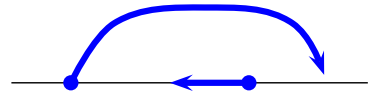
Fig. 4.6 In one dimension, two points cannot cross through each other without hitting each other. But if we allow the points to move in two dimensions they can get around each other without touching. This is supposed to show you that one-dimensional world-lines cannot form knots in four-dimensional space.
