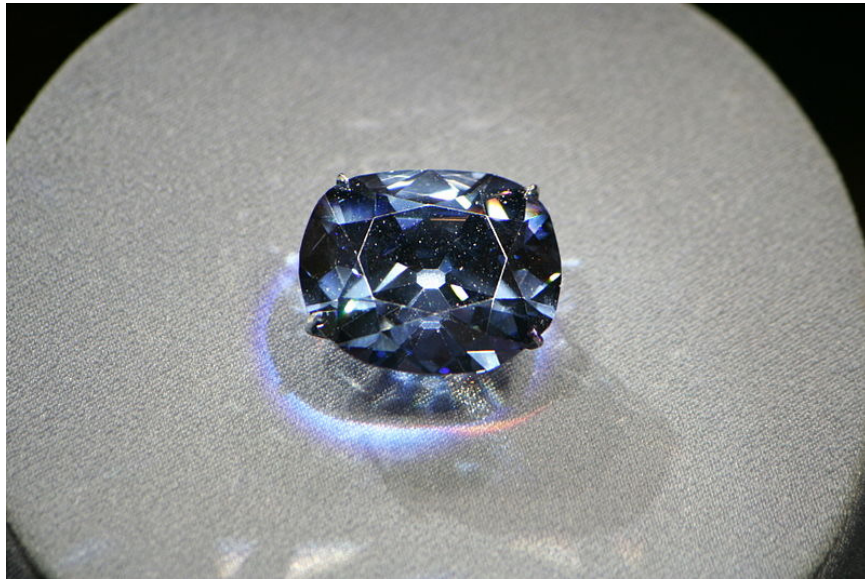
Hope Diamond (Blue) Roughly 1 Boron impurity per 10^7 carbon. Estimated current value = 250 Million $
