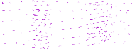
Figure 5.1: Compression Waves = Longitudinal Phonon
