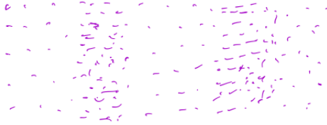
Figure 5.1: Compression Waves = Longitudinal Phonon
