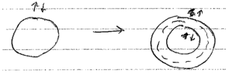
Figure 9.8: To determine spin susceptibility, we increase the size of the fermi surface for spin up and reduce the size of the fermi surface for spin down
