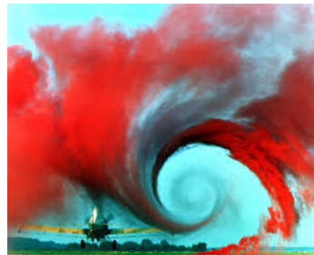
Figure 5: Vortices around an aircraft.
