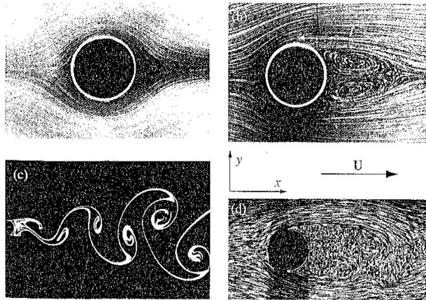
Figure 1: Flow over a cylinder for different Reynolds numbers. (a)  $Re=0.16$ , almost symmetric, (b)  $Re=26$ , eddies behind cylinder, fixed in space, (c)  $Re=200$ , Bénard - von Karman vortex street, (d)  $Re=8000$ , turbulent wake.
