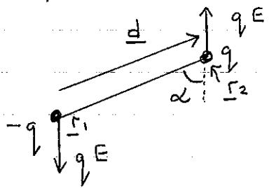
$$\begin{aligned} \underline{\tau} &= q \underline{E} \cdot d \sin \alpha = p E \sin \alpha \\ \underline{\tau} &= \underline{p} \times \underline{E} \\ \text{out of paper} && \text{right magnitude} \\ && \text{and out of paper} \end{aligned}$$
