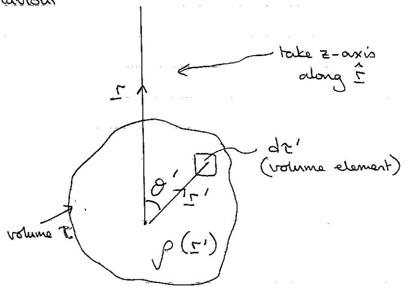
$$V(\Sigma) = \int_V \frac{\rho(\Sigma') d\Sigma'}{4\pi\epsilon_0 |\Sigma - \Sigma'|}$$
