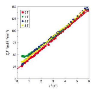
Heat capacity  $\sim aT + bT^3$
