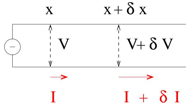
*voltage and current signals propagate along the line*
