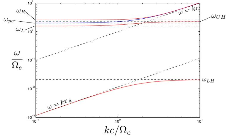
FIGURE 4. Cold plasma waves with perpendicular propagation for an electron-proton plasma ( $Z = 1$ ,  $m_i/m_e = 1836$ ) with  $\omega_{pe}/\Omega_e = 2$ . The ordinary mode is represented as a blue line, and the extraordinary mode as red lines. For comparison, we plot the frequencies  $\omega_L$ ,  $\omega_R$ ,  $\omega_{UH}$  and  $\omega_{LH}$  and the dispersion relations for light ( $\omega = kc$ ) and Alfvén waves ( $\omega = kv_A$ ) as dashed lines.
