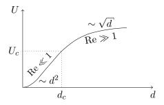
This formula applies for slow velocities, large viscosities or low densities/small bubbles. Thus, we can once again apply the force balance equation with the Archimedes force
