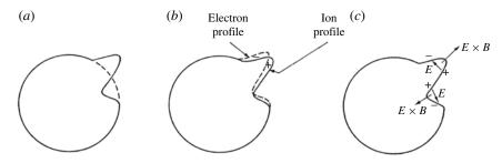
FIGURE 49. Development of the flute instability in a mirror machine (from Taylor 1968); see text for details.
