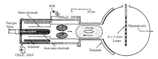
FIGURE 43. Schematic of spheromak injection into ENCORE tokamak at Caltech. (Reproduced with permission from Brown & Bellan (1990). Copyright 1990, AIP Publishing LLC.)
