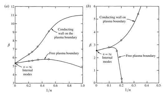
FIGURE 61. Critical  $\beta$  as a function of 1/n for a configuration with (a) R/a = 3.5,  $\kappa = 1.65$ ,  $\delta = 0.25$ ,  $\alpha = 1.4$  and 1.0 < q < 3.0 and (b) R/a = 4.6,  $\kappa = 1.0$ ,  $\delta = 0$ ,  $\alpha = 2$  and 1.04 < q < 1.58. (Reproduced with permission from Todd *et al.* (1979).)
