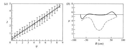
FIGURE 33. (a) Poloidal current versus poloidal flux and (b) measured profile of  $\mu(r)$  in S-1 spheromak. (Reproduced with permission from Hart *et al.* (1986). Copyright 1986, AIP Publishing LLC.)
