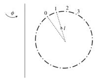
FIGURE 5. Poincaré plot generated by following a magnetic field line through many circuits around the torus.
