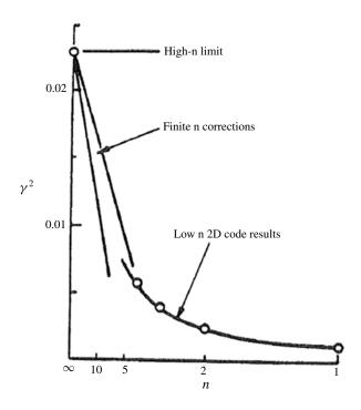
FIGURE 59. Variation of growth rate with toroidal mode number from direct MHD simulation for an unstable JET configuration, with central safety factor  $q_0 = 0.75$ , edge safety factor  $q_a = 6.4$  and average  $\beta = 0.045$ . (Reproduced with permission from Sykes *et al.* (1979).)
