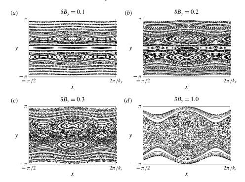
FIGURE 12. Illustration of the break-up of magnetic surfaces in the presence of multiple perturbations with increasing strength: (a)  $\delta B_y = 0.1$ ; (b)  $\delta B_y = 0.2$ ; (c)  $\delta B_y = 0.3$ ; (d)  $\delta B_y = 1.0$ .
