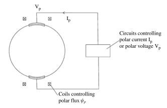
FIGURE 37. Set-up to control relaxed state of flux core spheromak externally.
