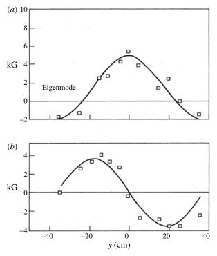
FIGURE 32. Magnetic field profiles in the BETA II spheromak. (a) Poloidal field and (b) toroidal field. Experimental measurements are shown as squares; the solid line is the theoretical prediction. (Reproduced with permission from Turner *et al.* (1983). Copyright 1983, AIP Publishing LLC.)
