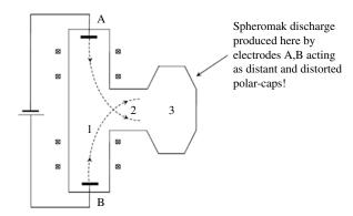
FIGURE 41. Illustration of kinked Z-pinch source.
