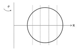
FIGURE 3. Constant pressure surfaces in a purely toroidal field.
