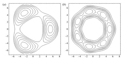
FIGURE 11. Magnetic surfaces resulting from a helical perturbation with (a) m = 3 and (b) m = 7.
