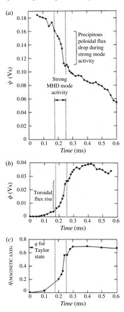
FIGURE 34. Time dependence of magnetic fields in S-1 spheromak – see text for details. (Reproduced with permission from Janos *et al.* (1985*a*).)
