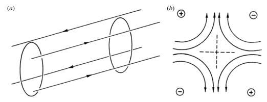
FIGURE 51. (a) Mirror machine stabilisation by Ioffe bars and (b) the resulting magnetic field (from Taylor 1968).
