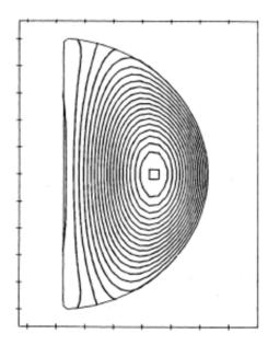
FIGURE 38. Calculated field in a flux core spheromak,  $\mu a = 4.09$  (from Taylor 1986).
