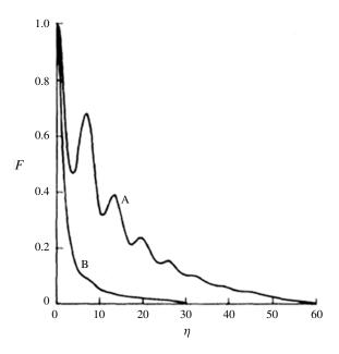
FIGURE 57. Marginally stable eigenfunctions for (A) low shear, s = 0.1, and (B) high shear, s = 0.7 (from Connor *et al.* 1978).
