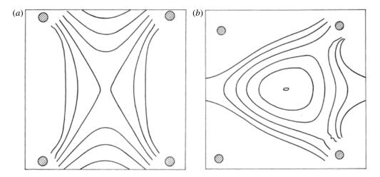
FIGURE 52. Magnetic isobars in a stabilised minimum-B mirror device for (a) small current in the stabilising rods and (b) large current in the rods (from Taylor 1968).
