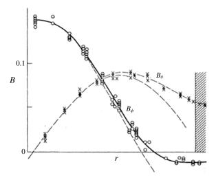
FIGURE 19. Comparison of experimental magnetic field profiles in the quiescent state of the toroidal pinch HBTX-1A to the theoretical expressions (8.4). (Reproduced with permission from Bodin (1984).)
