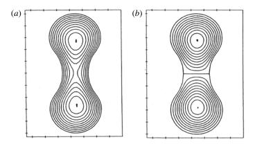
FIGURE 27. Relaxed profiles in the multipinch: (a) primitive relaxed state, with  $\mu a = 1.5$  and (b) lowest eigenfunction, with  $\mu a = 2.21$ . (Reproduced with permission from La Haye et al. (1986).)
