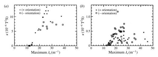
FIGURE 42. Spheromak figure of merit  $\kappa$  versus  $\lambda_e \equiv \mu$ . (Reproduced with permission from Fernández *et al.* (1989). Copyright 1989, AIP Publishing LLC.)
