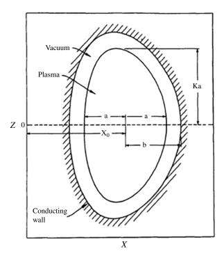
FIGURE 60. Geometry used to study ballooning stability. (Reproduced with permission from Todd *et al.* (1979).)
