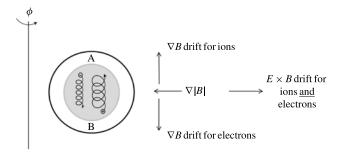
FIGURE 2. Particle motion in a toroidal field.
