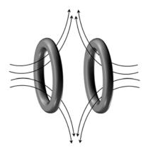
FIGURE 50. Sketch of spindle cusp configuration.
