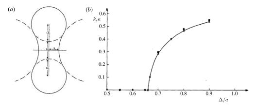
FIGURE 28. (a) Idealised multipinch and (b) toroidal wavenumber corresponding to the lowest eigenvalue as a function of  $\Delta$ . (Reproduced with permission from Gimblett *et al.* (1987). Copyright 1987, AIP Publishing LLC.)
