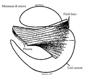
FIGURE 53. Schematic of the tennis ball coil and field lines. (Reproduced with permission from Post (1987).)
