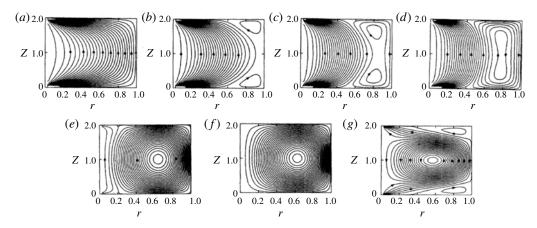
FIGURE 39. Evolution of analytic field profiles in an idealised flux core spheromak at various values of  $\mu a$ : (a)  $\mu a = 0.001$ , (b)  $\mu a = 2.25$ , (c)  $\mu a = 2.70$ , (d)  $\mu a = 3.00$ , (e)  $\mu a = 4.00$ , (f)  $\mu a = 4.14$  and (g)  $\mu a = 5.00$ . (Reproduced with permission from Turner (1984). Copyright 1984, AIP Publishing LLC.)
