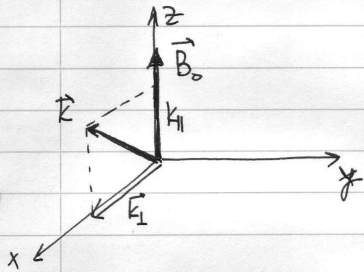
$$\left\{ \begin{array}{l} \omega^2 \vec{\zeta}_x = c_s^2 k_{\perp} (k_{\perp} \vec{\zeta}_x + k_{\parallel} \vec{\zeta}_{\parallel}) + V_A^2 k^2 \vec{\zeta}_x \\ \omega^2 \vec{\zeta}_y = V_A^2 k_{\parallel}^2 \vec{\zeta}_y \\ \omega^2 \vec{\zeta}_{\parallel} = c_s^2 k_{\parallel} (k_{\perp} \vec{\zeta}_x + k_{\parallel} \vec{\zeta}_{\parallel}) \end{array} \right.$$
