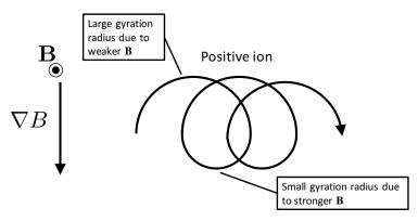
FIGURE 3. The  $\nabla B$  drift is the result of the radius of gyration changing because of the magnetic field magnitude variations along the path of the particle.
