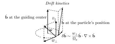
FIGURE 4. Sketch of the magnetic field direction at the position of the particle and at the position of the guiding center.
