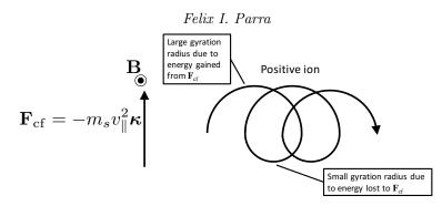
FIGURE 2. The curvature drift is the result of the centrifugal force (see figure 1) accelerating and decelerating the particle in its gyration, and consequently changing the radius of gyration.
